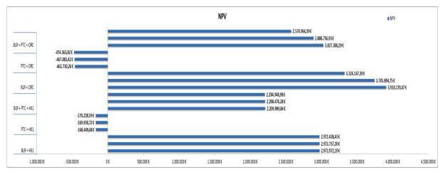
*Figure 65 - Comparison of net present values between different PowerStation combinations.*
