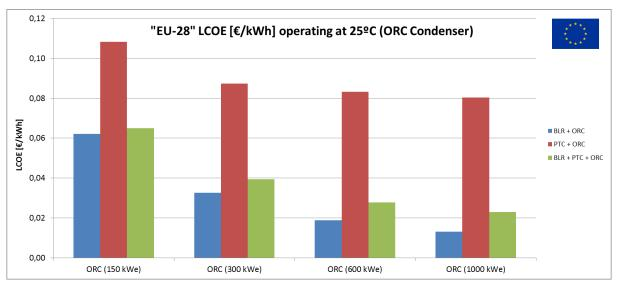
Figure 93 – LCOE for EU28 in function of ORC scaling
