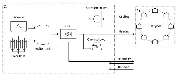
Figure 44 – Single line diagram of the energy system.
