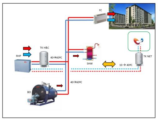
Figure 2 – Block of flats with FLEXYNETS.
