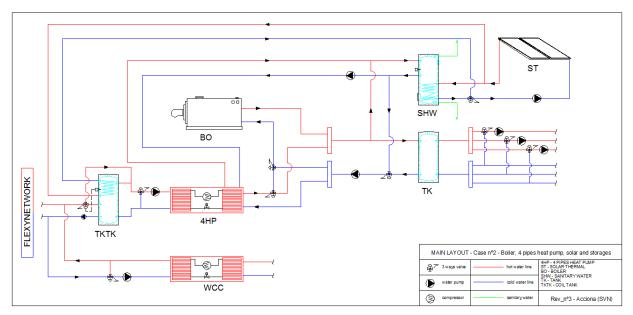
Figure 105 – Global P&ID for 4 pipes domestic sub-station
