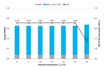
*Figure 29 - Yearly energy balance for residential substations: new/renovated ("45") SFH buildings for the location of London.*
