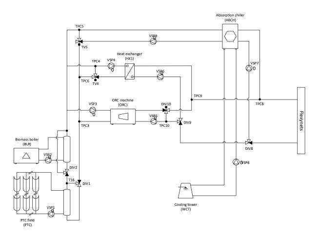
Figure 45 – Layout of power station.
