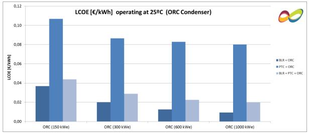
In the following picture, it is represented the variation of LCOE according to PowerStation scaling up:
