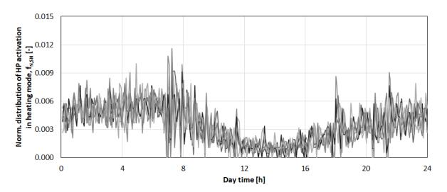
Figure 41 – Normalized distribution of heat pump activation in heating mode for the month of January for different FLEXYNETS temperatures (Building: SFH, Location: Rome).
