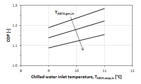
Figure 49 - Thermal COP of the absorption chiller as a function of the chiller water inlet temperature for different generator inlet temperatures (165, 170, 175 °C, increasing along the arrow direction) at 28°C inlet condenser temperature.
