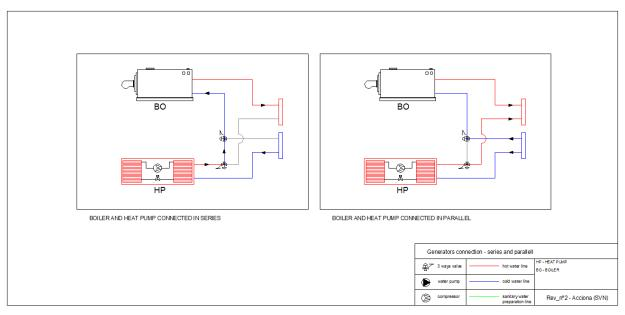
Figure 102 – Detail of connection boiler with HP
