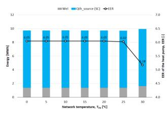
Figure 37 - Yearly energy balance for residential substations: new/renovated ("45") s-MFH buildings for the location of Stuttgart.
