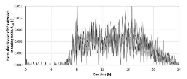
Figure 43 – Normalized distribution of heat pump activation in SC mode for the month of July for different FLEXYNETS temperatures (Building: SFH, Location: Rome).
