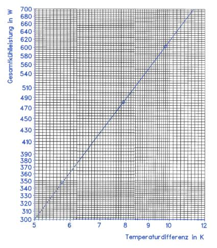
Figure 84 – Characteristic curve of the radiant ceiling TRIPAN<sup>®</sup>.
