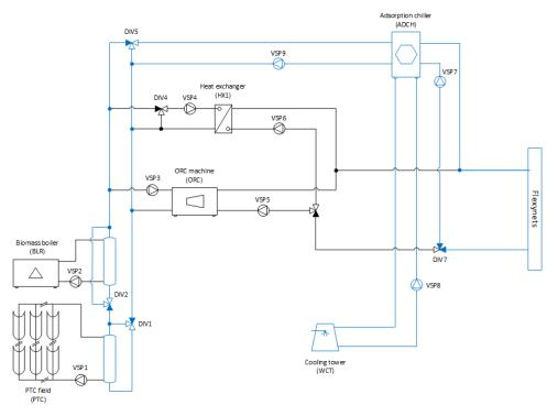
Figure 53 – Working scheme Sc3.
