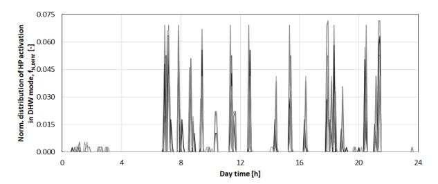
Figure 42 – Normalized distribution of heat pump activation in DHW mode for the month of January for different FLEXYNETS temperatures (Building: SFH, Location: Rome).
