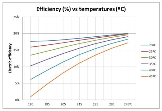
Figure 48 - ORC electrical efficiency of ORC unit as a function of oil inlet temperature for different condensing water temperatures.
