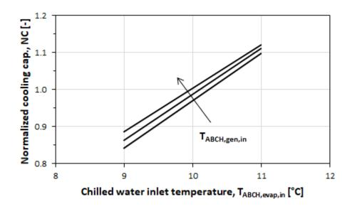
Figure 50 – Normalized cooling capacity of the absorption chiller as a function of the chiller water inlet temperature for different generator inlet temperatures (165, 170, 175 °C, increasing along the arrow direction) at 28°C inlet condenser temperature.
