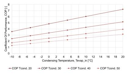
Figure 22 - Coefficient Of Performance for a Water to Water Heat Pump in winter mode as a function of the ambient air and the inlet water temperature at the condensing side.
