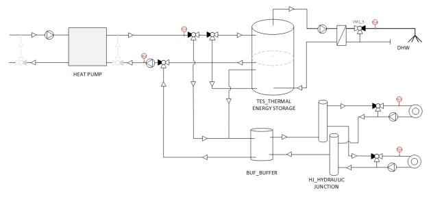
Figure 21 - Schematic of the hybrid system used for the SFH.
