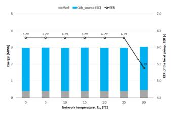
Figure 33 - Yearly energy balance for residential substations: new/renovated ("45") SFH buildings for the location of Rome.
