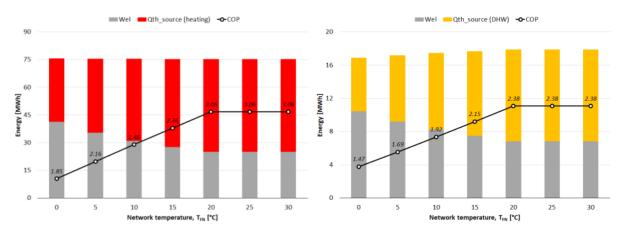
Figure 36 – Yearly energy balance for residential substations: existing ("EX") s-MFH buildings for the location of Stuttgart.
