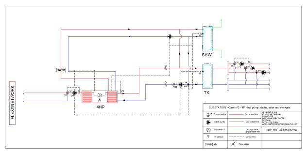
Figure 106 – Simplified lay-out for software implementation (4 pipes HP)
