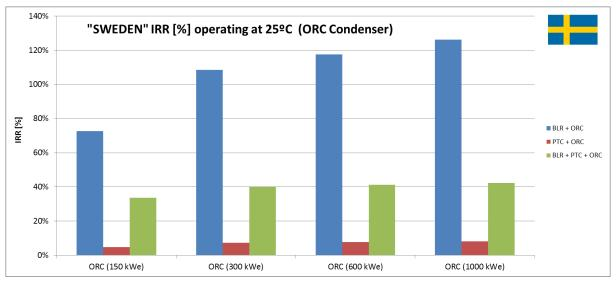
Figure 100 – IRR for SWEDEN in function of ORC scaling
