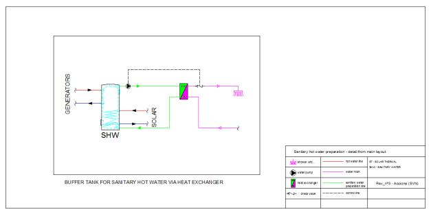
Figure 103 – Detail of SHW production
