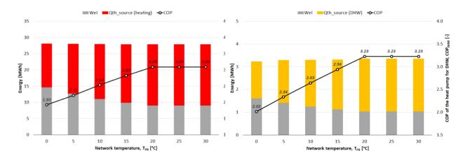
Figure 30 – Yearly energy balance for residential substations: existing ("EX") SFH buildings for the location of Stuttgart.
